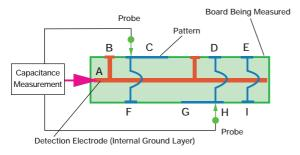
Capacitance measurement is also possible using vacuum clamping.
