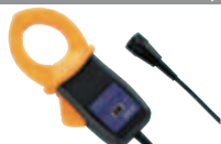
CLAMP ON SENSOR 9272-10 20A/ 200A AC φ46mm(1.81") POWER SUPPLY: 9555-10
