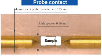
Shape of probe tip: 60° cone
