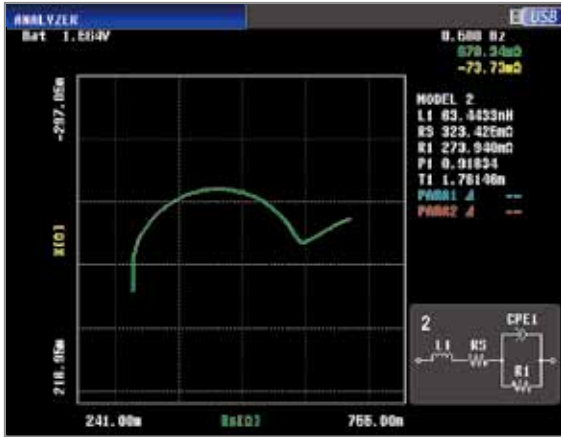
Cole - Cole plot screen (manganese battery)
