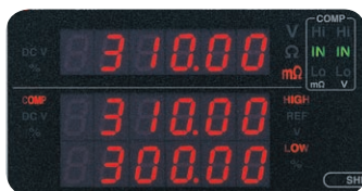
Resistance comparator settings
