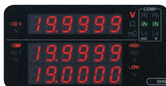
Voltage comparator settings
